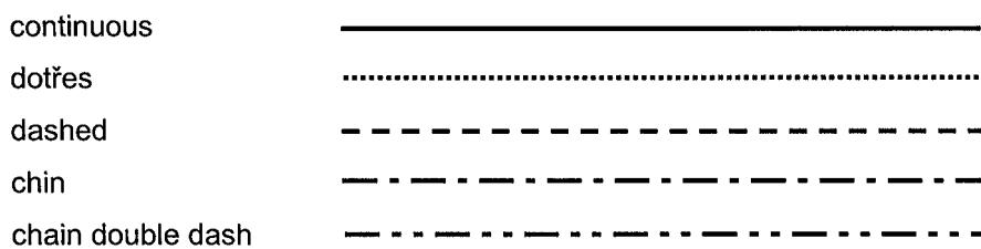
**Figure 1 – Illustration of predefined curve fonts**
