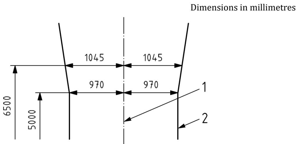
**Figure G.3 — Kinematic reference profile for 25 kV pantographs in the raised position for gauges BE1, BE2 and BE3**
