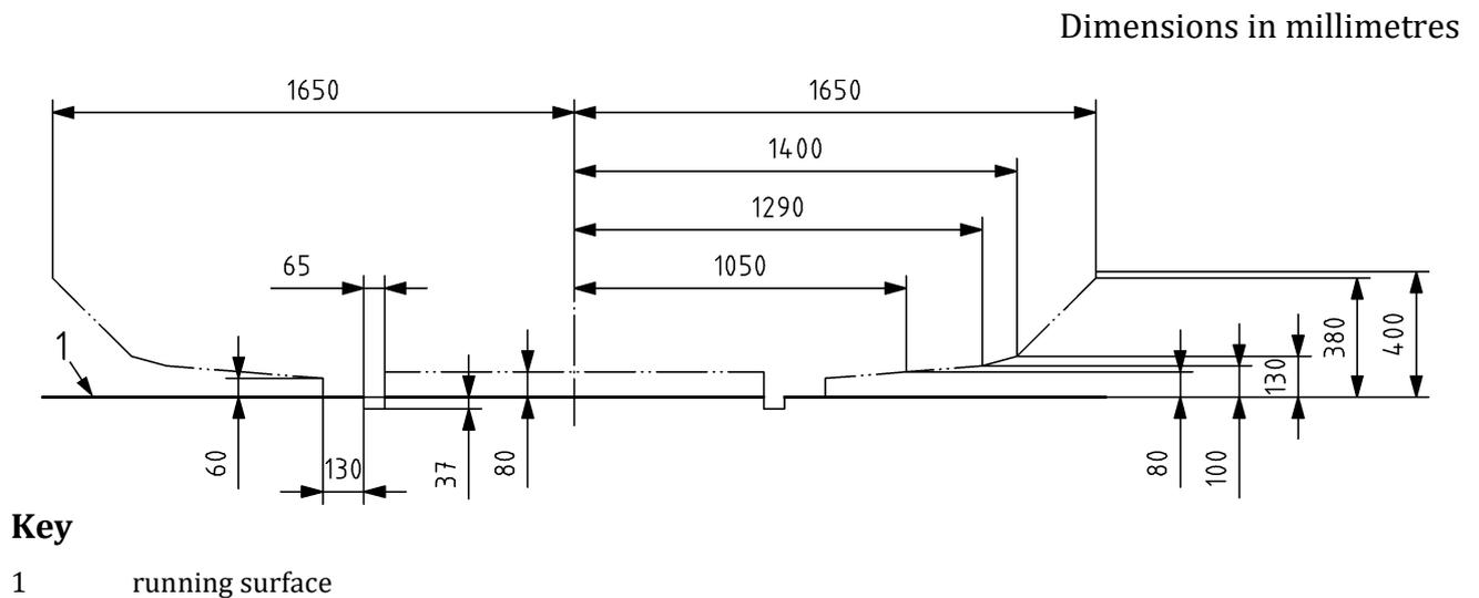
**Figure C.18 — Lower zone not compatible with the marshalling humps**
