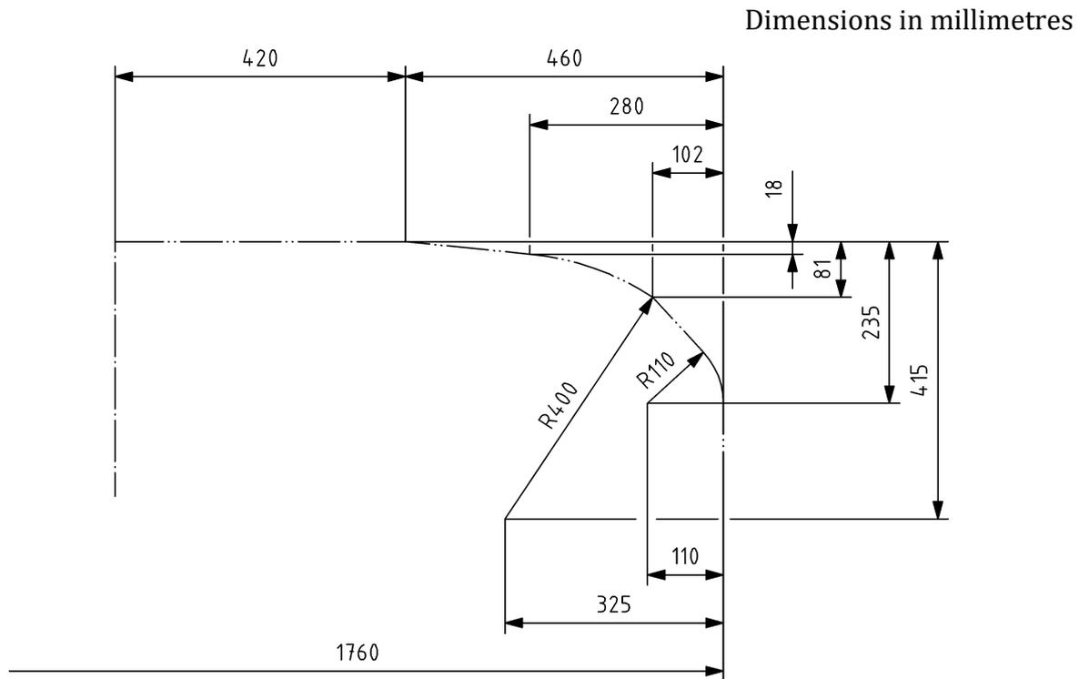
**Figure G.1 — Head with 1,760 m width**
