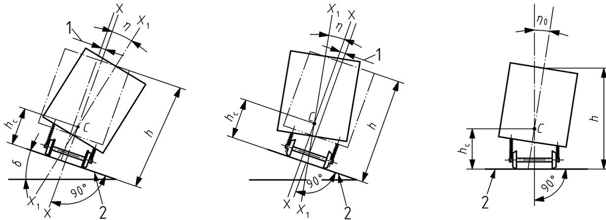
**a) Stationary vehicle on a canted curve**
