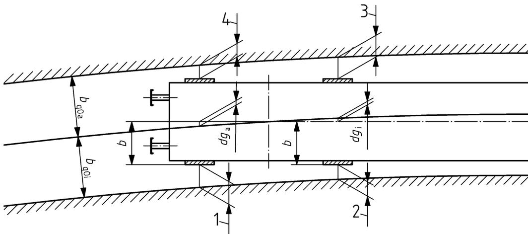
**Figure H.1 — Illustration of the conventional gap**
