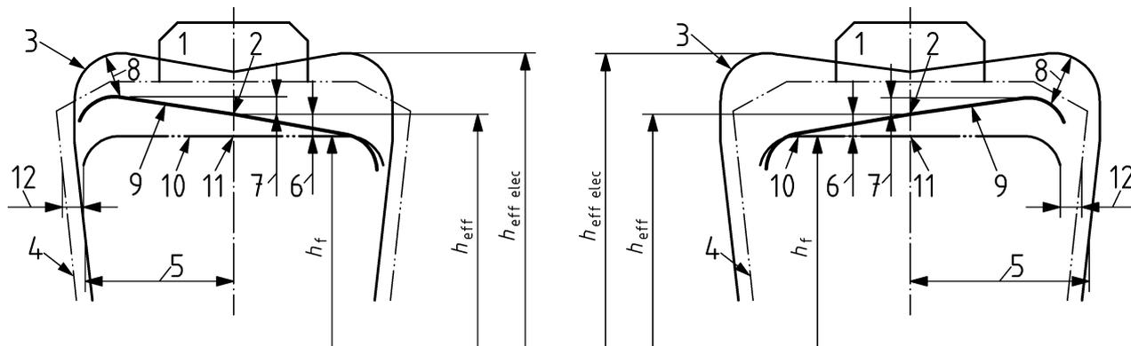
**a) Pantograph fitted with insulating horns      b) Pantograph fitted with non-insulating horns**
